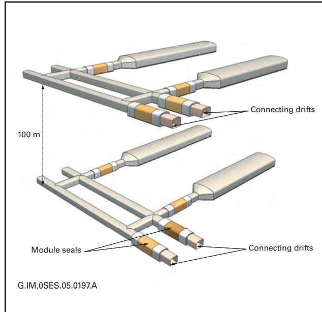
**Principle of locating B waste disposal cells**
