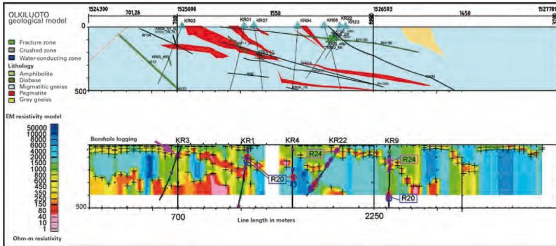
**Geological cross-section and resistivity of the electromagnetic line (200 metres transmitter-receiver spacing, broadside array)**
