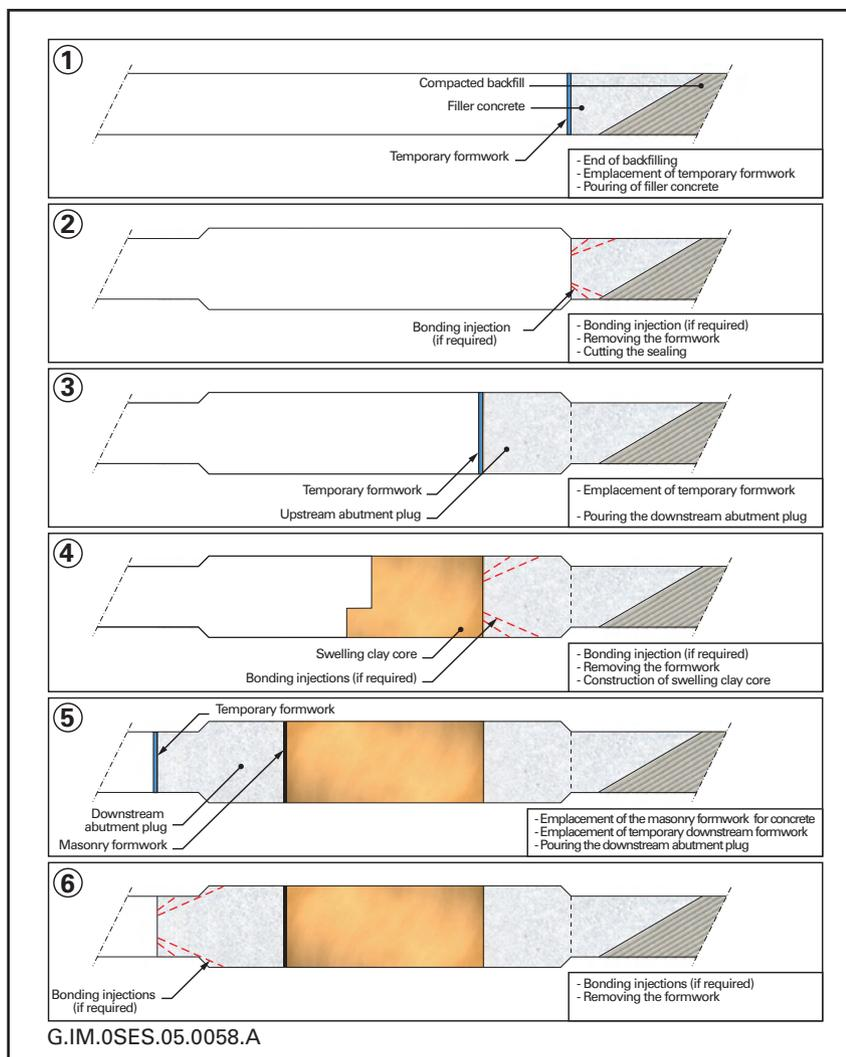
**Principle of the seal construction**
