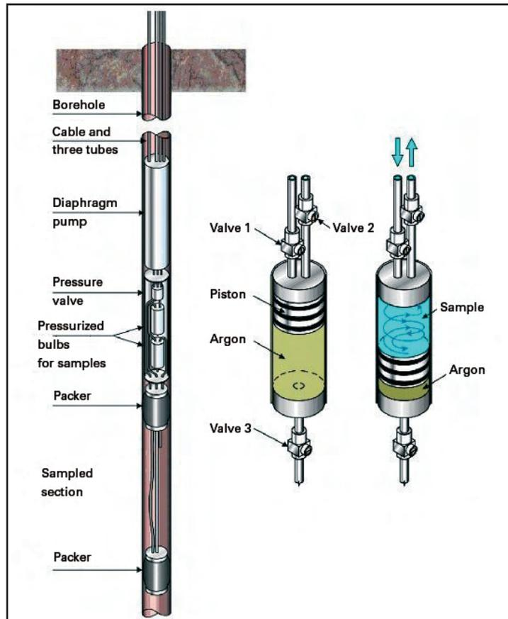
**PAVE borehole fluid sampling system developed in Finland (Posiva data)**
