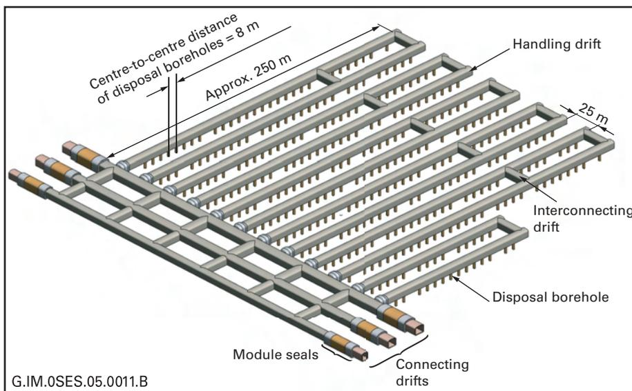
**Typical architecture of a C waste repository module**
