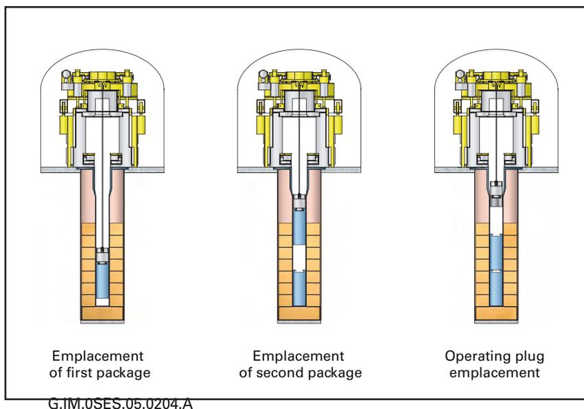
***C waste repository: emplacement and possible retrieval of packages in disposal borehole***
