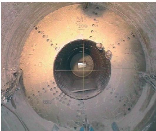
**b/ When the structure has resaturated, the joints between bricks are no longer visible, as a result of the swelling within the buffer**
