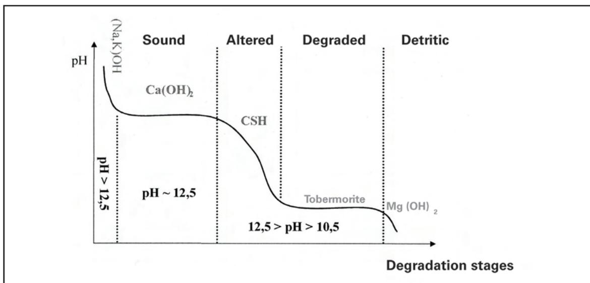
**Stages in the concrete degradation process**
