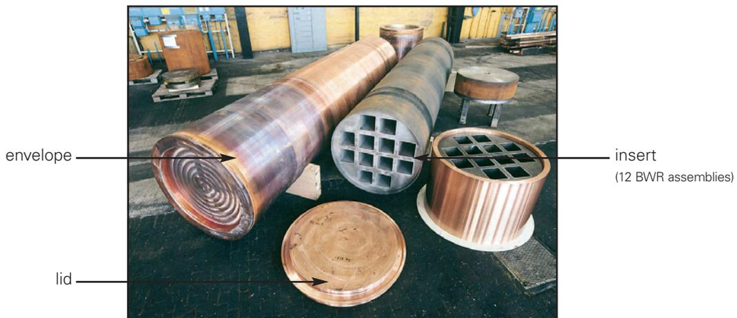
**View of the copper envelope and insert for BWR assemblies (source SKB)**
