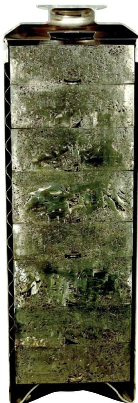
*Cut-away model of a CSD-C container, showing the stack of wafers*
