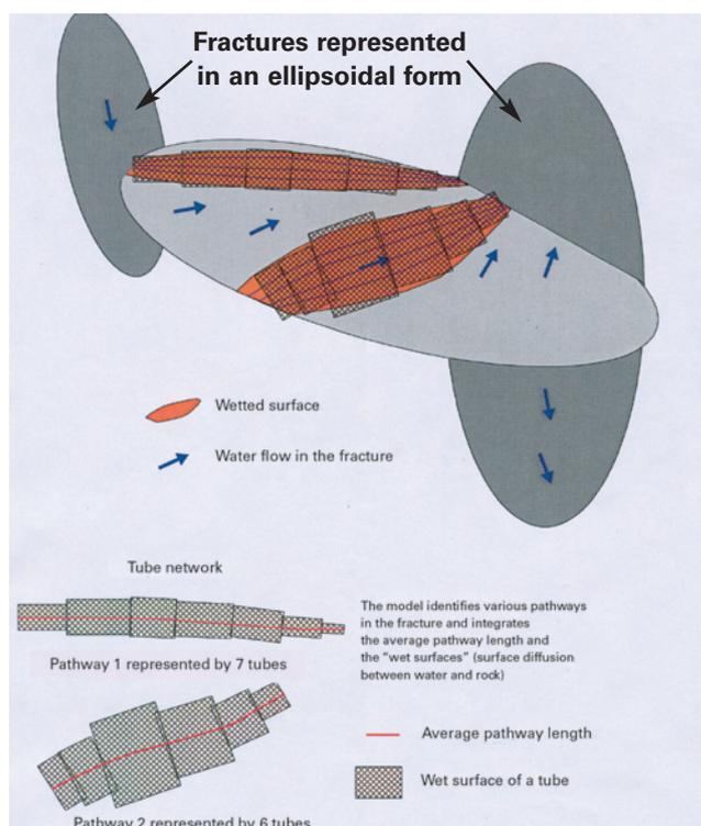
***Tube model of water and radionuclides pathway in a fracture***
