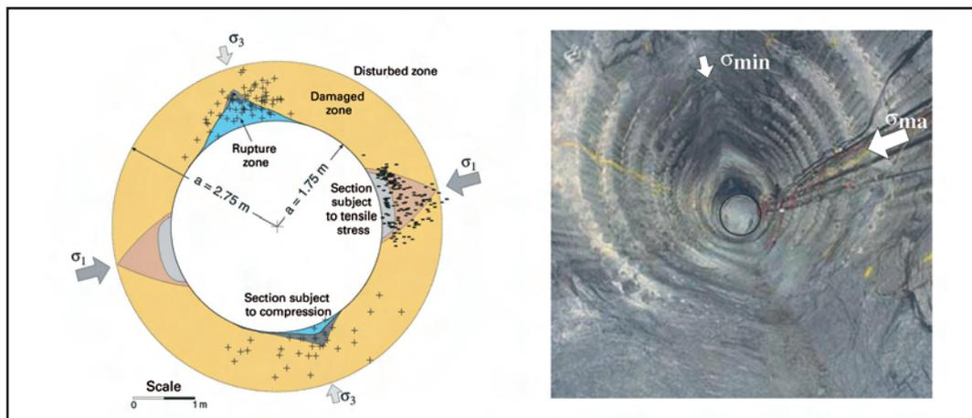
**Lac du Bonnet underground laboratory in Canada: damage to the granite wall of a circular drift subjected to a highly anisotropic stress configuration**
