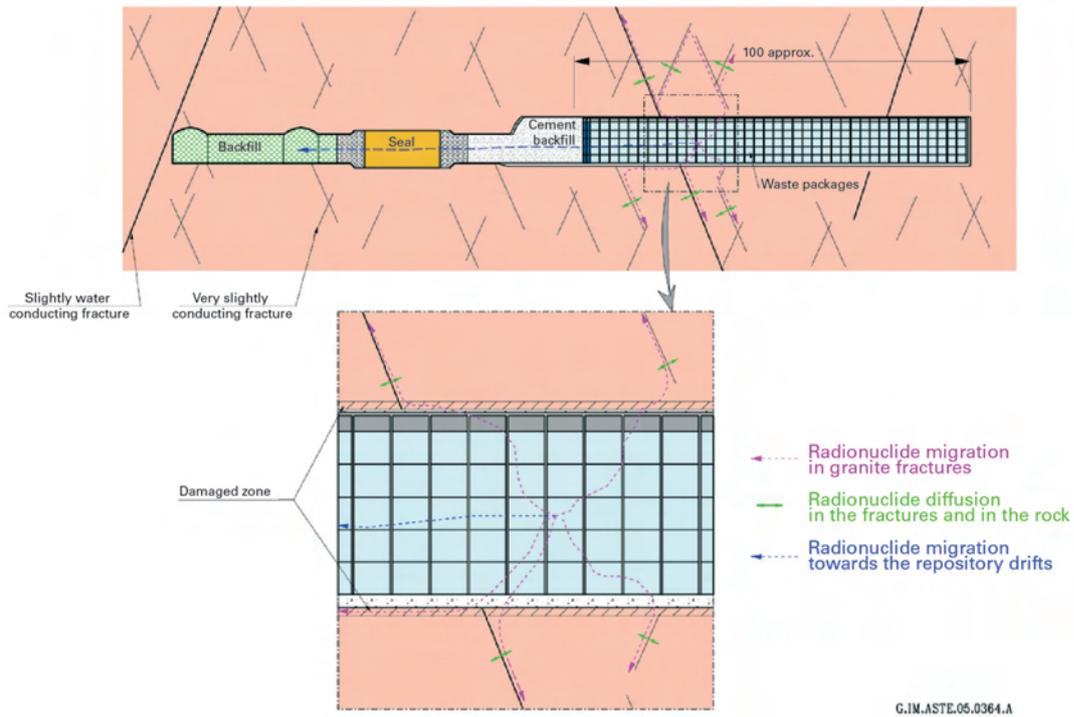
**Scheme of the migration of radionuclides in the B waste disposal tunnels**
