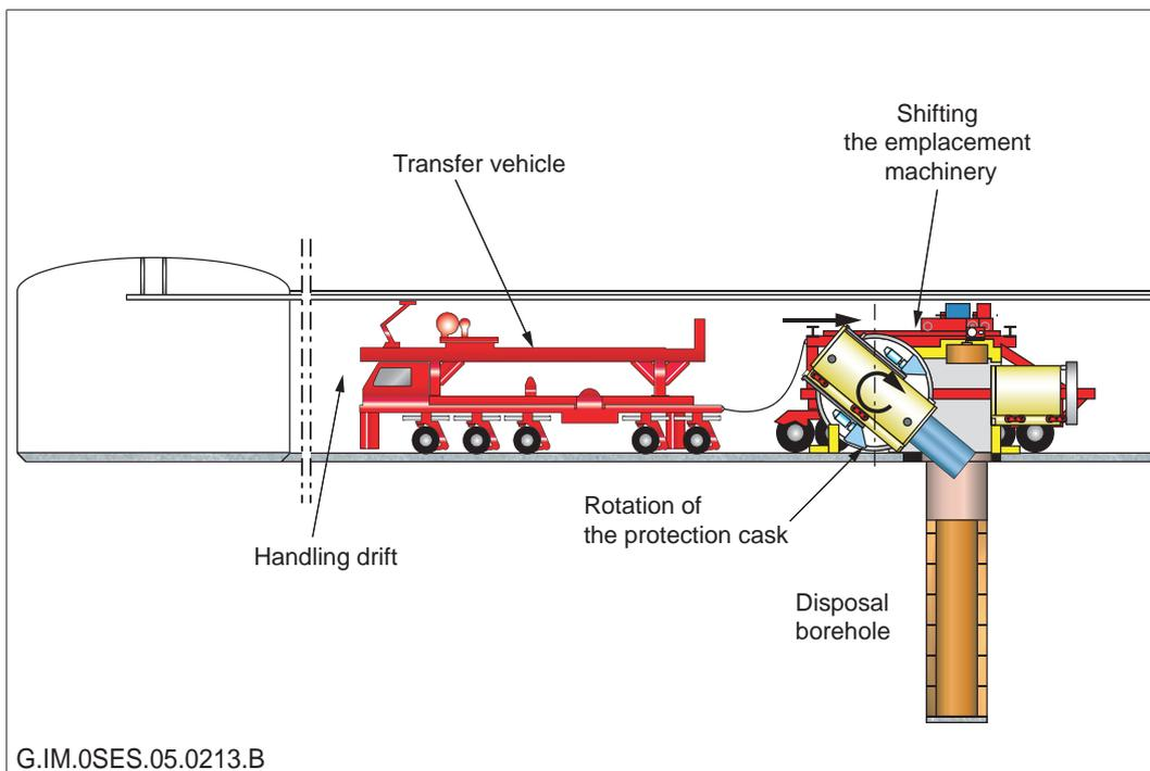
**The KBS-3 concept (Sweden): principle of emplacing spent fuel containers in the disposal borehole (pit)**
