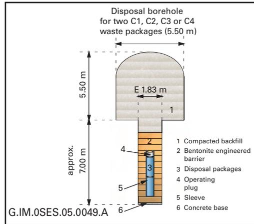
**•The C waste disposal packages: a carbon steel overpack**
