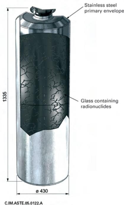
**Diagram of an R7T7 vitrified C waste primary package**
