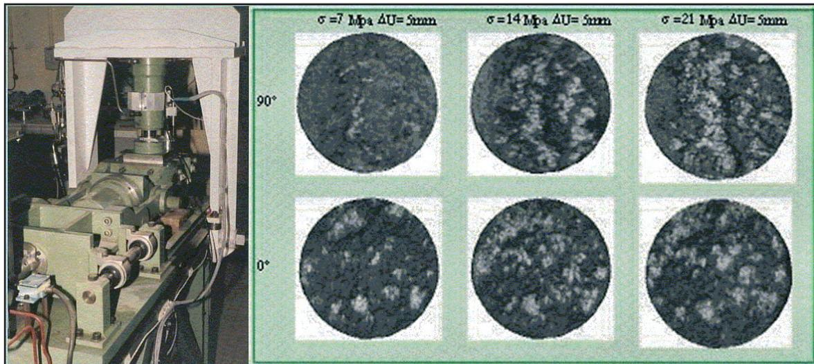
**Equipment used for shear tests on fracture samples in granite and photos of post-shear fractures surfaces (5 min) (Riss and al, 1997)**
