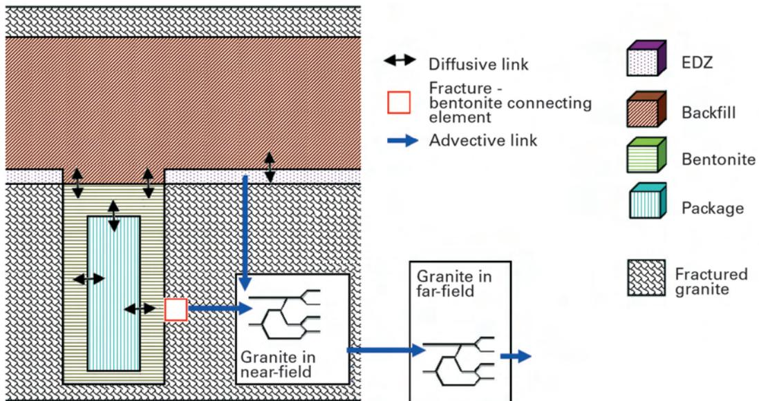
**Modelling the transfers in a C waste disposal cell (DFN approach in granite)**
