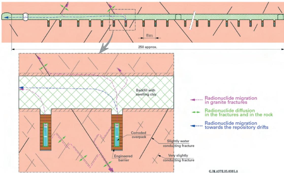
**Scheme of the migration of radionuclides in the C waste disposal boreholes and the handling drifts**
