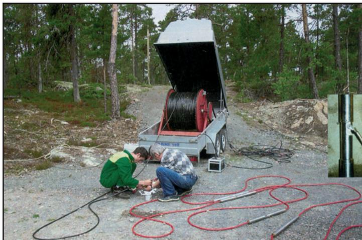
**Seismic source (left) and set of eight geophones before they were lowered down a borehole (right)**
