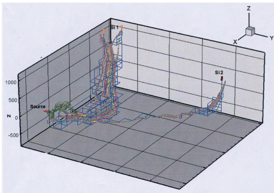
*Performance calculations of a repository in a granite medium: "tube" model of radionuclides pathways between the repository (source) and the outlets (Si1 and Si2)*
