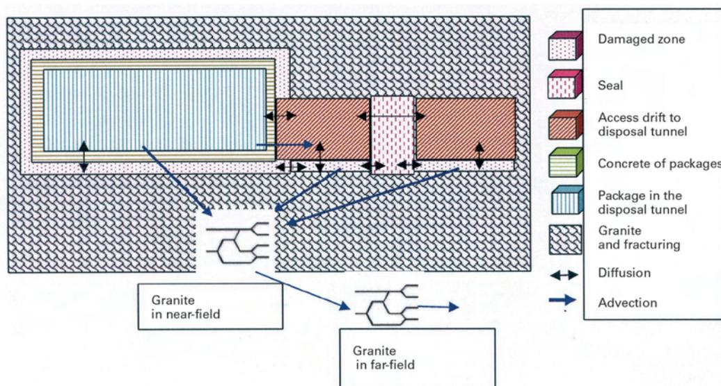
**Model of the B waste disposal tunnel and transfer regimes (DFN approach in granite)**
