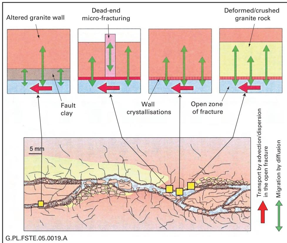
**Conceptual model of fractures and transport phenomena**
