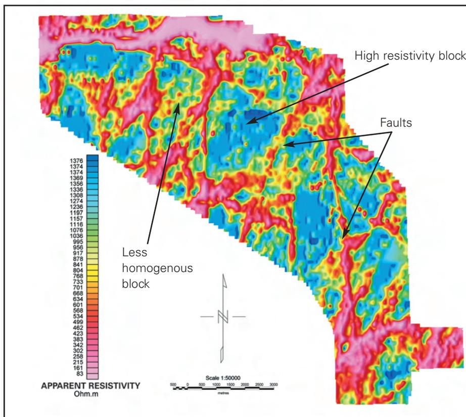
**Airborne resistivity map showing the separation of a granite massif into “blocks” by faults (Cogema data)**
