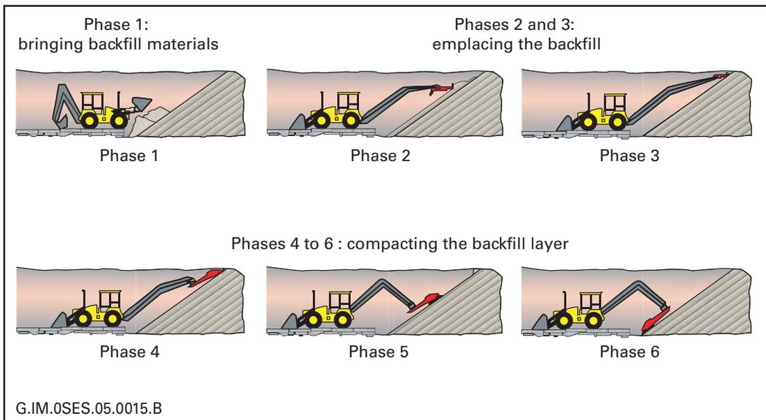
**Principle of installing a low permeability backfill**
