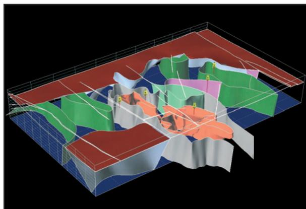
**Left: visualisation of faults and cross sections with the RVS developed by SKB (Sweden).**
