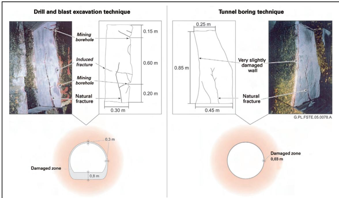
**Damaged zone on the drift wall ("ZEDEX" experiment at the Äspö laboratory)**
