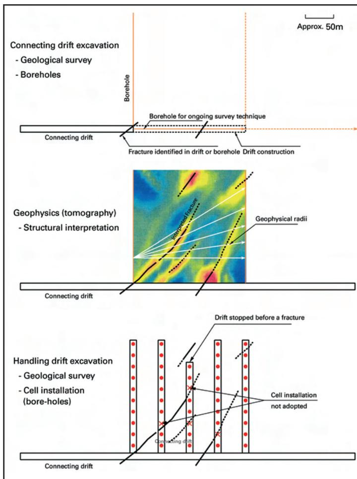
**Principle for determining the degree of fracturing through the ongoing method (as excavation works progress)**
