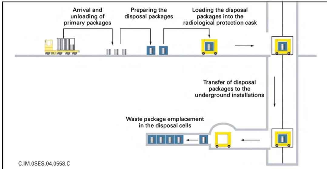
**Diagram of the principle of nuclear operation of the repository**
