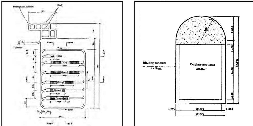
**General architecture of a deep TRU waste repository in crystalline rocks and disposal tunnel for bitumised or low-level waste (Japan)**
