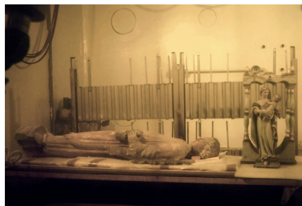
Disinfection of a mummy by (cobalt-60) irradiation. Source rods can be seen in the background
