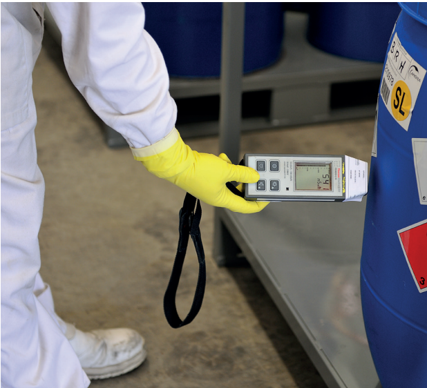
Radiological monitoring: radiation measurement on a waste package
