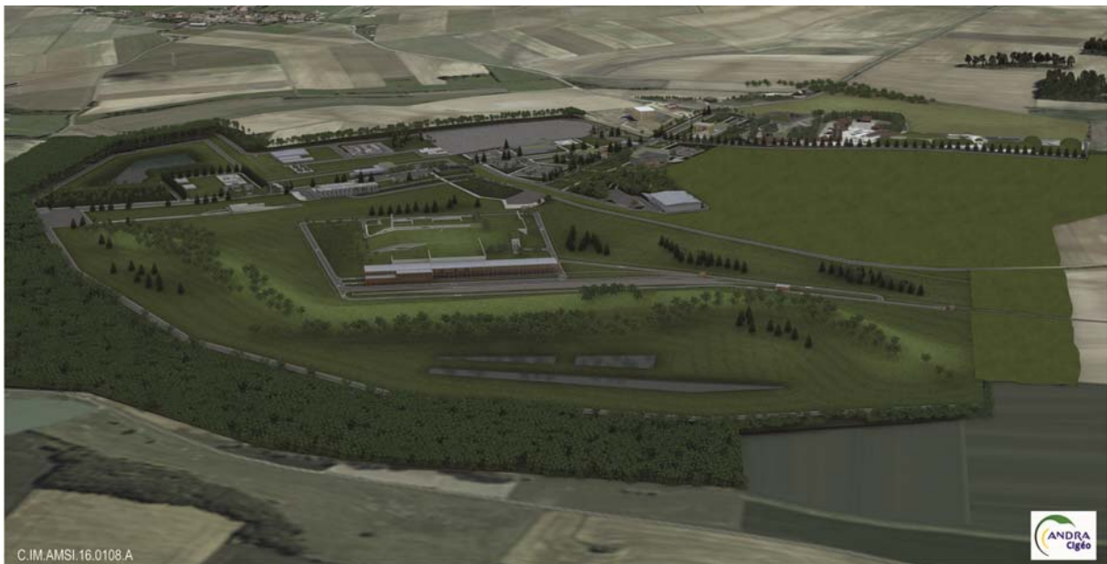
Figure 2-7 3D view of the surface structures in the zone reserved for the receipt, inspection, and preparation of waste packages to be built during the T1 phase (ramp zone) (based on the basic engineering design).
