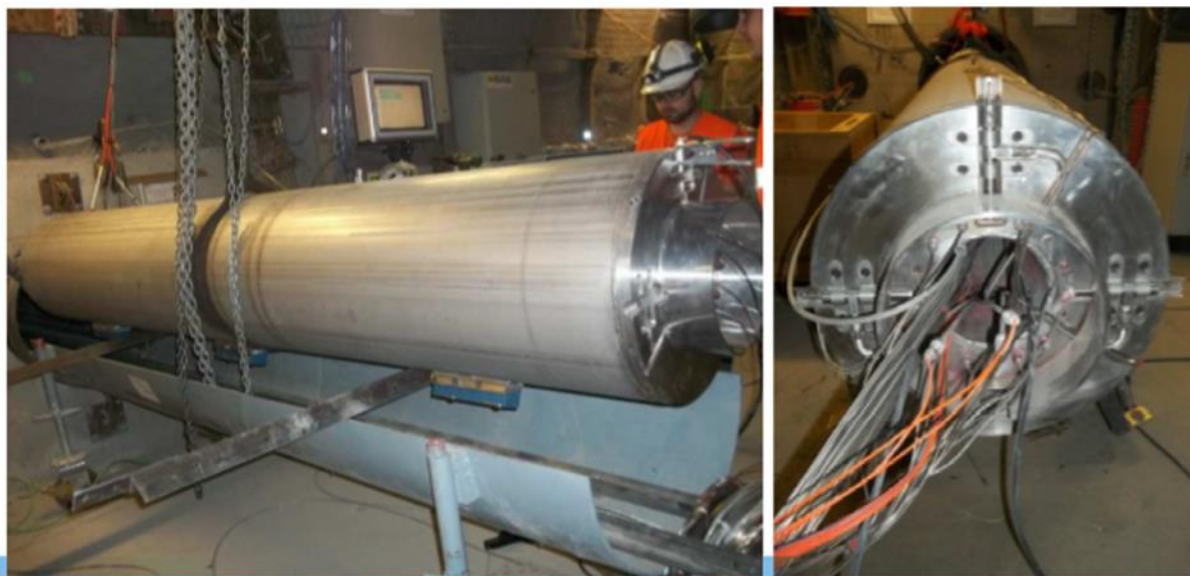
Figure 28 View of a heater element when it is installed left) – View of a heater/sleeve distance variation sensor section (right)
