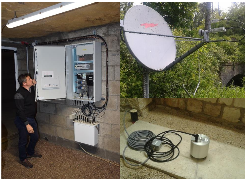
Figure 3 Components of a seismic monitoring station in the RES network (3-component seismometer, cable and IT cabinet with PC, digitizer, router, modems) and Vsat satellite dish
