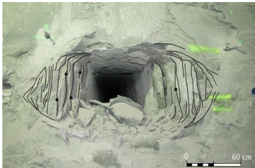
Figure 7 Fracture network around cell ALC3005
