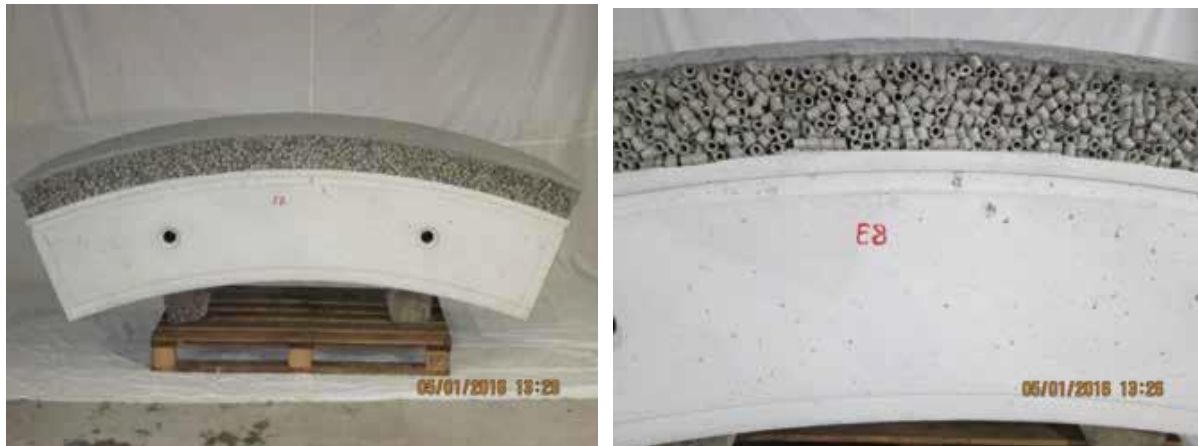
Figure 33 VMC prototype (left) and its compressible material coating (right) for GVA test drift
