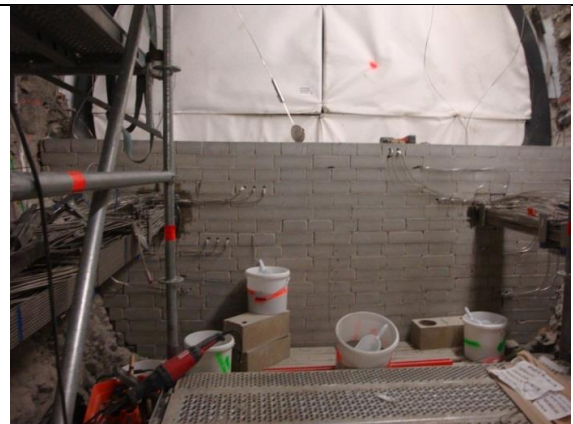
Placement of blocks and installation of sensors in the core
