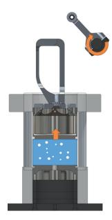
▶ Principle of impact-assisted cavitation: a mechanical arm drives a piston and forcefully releases it to impact the liquid. A shock wave is produced, followed by resonance waves, which creates cavitation bubbles of varying size.
