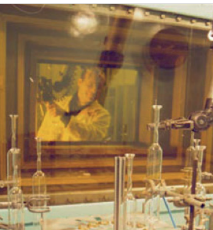
► Fig.2. The IRSN IRMA gamma irradiation facility ( ^{60}\text{Co} ) to test the behaviour of optical fibres under irradiation
