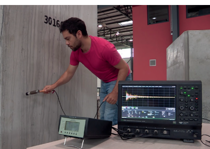
► Mechanical stress test on a concrete container.
