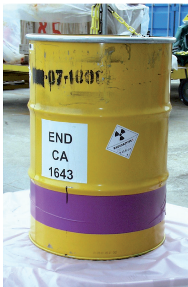
► 200 L metal drum used for conditioning cemented and other waste.
