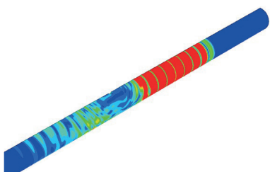
► Simulation of guided wave propagation in a tube
