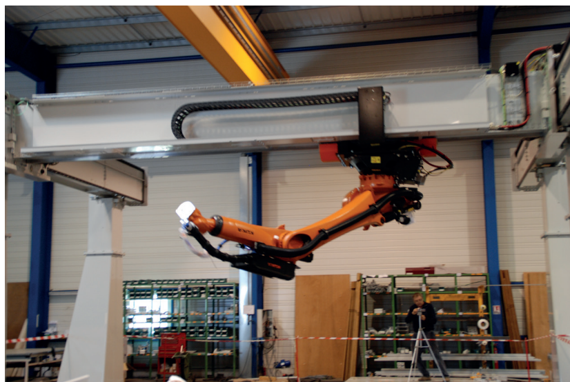
► Gantry equipped with 2 robots (14 controlled axes) with a tool changer adapted to the different CND technologies used to control the integrity of the radioactive waste containers - Lucas/Clemessy type configuration
