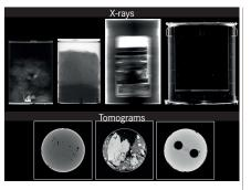
Example of high energy imaging produced in a permanent bunker on a dense package: X-rays and tomographic sections. Internal structures, material distribution and defects can be detected by these examinations.
