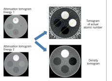
Simulation of a dual-energy tomographic examination, which makes it possible to determine the effective density and atomic number of the contents of a container.
