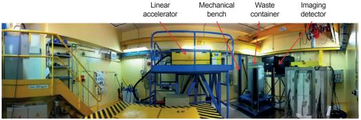
High energy tomograph at the CEA Cadarache CINPHONIE facility. The installation is located in an underground, shielded bunker. It can accommodate waste containers of up to five tons to produce tomographic or radiographic examinations with a spatial resolution of several millimetres.
