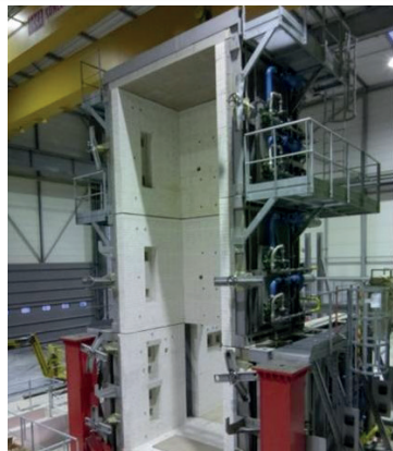
► CSTB Vulcain furnace (13.5 MW vertical furnace for testing elements that are 3 metres wide and up to 9 metres high with the possible application of mechanical loading)
