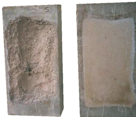
► Fire tested concrete blocks: left, plain concrete and right, polypropylene fibre reinforced concrete (Shuttleworth, 2001) 1
