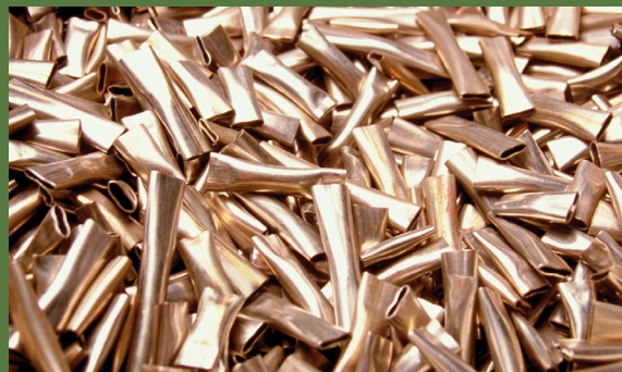
Hulls from the zirconium alloy cladding that covers fuel pellets
