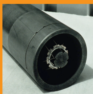
Graphite sleeve with wire locks
