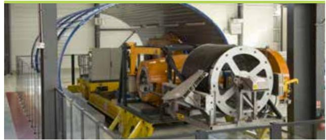
The Technological Space presents Cigéo through the exhibition of mock-ups and various robots and industrial prototypes built by Andra. The objective is to test and validate the technological concepts of this repository: concrete package container, handling system, etc.
