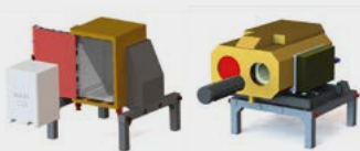
Transfer casks for ILW-LL and HLW packages
