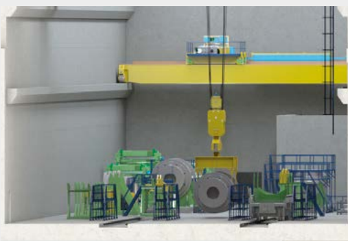
Reception and offloading of transport containers for ILW-LL waste packages
