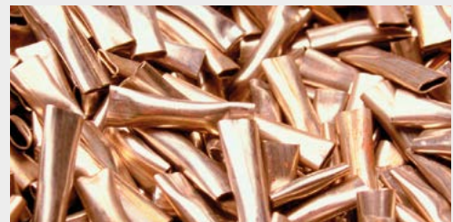
Sheared radioactive metal parts from spent fuel reprocessing
